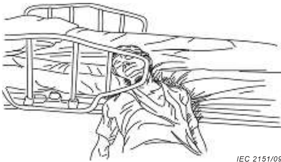
Figure AA.13 – Example of potential PATIENT entrapment in area B
