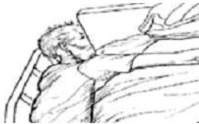
Figure AA.15 – Example of potential PATIENT entrapment in area C between SIDE RAIL and HEAD BOARD
